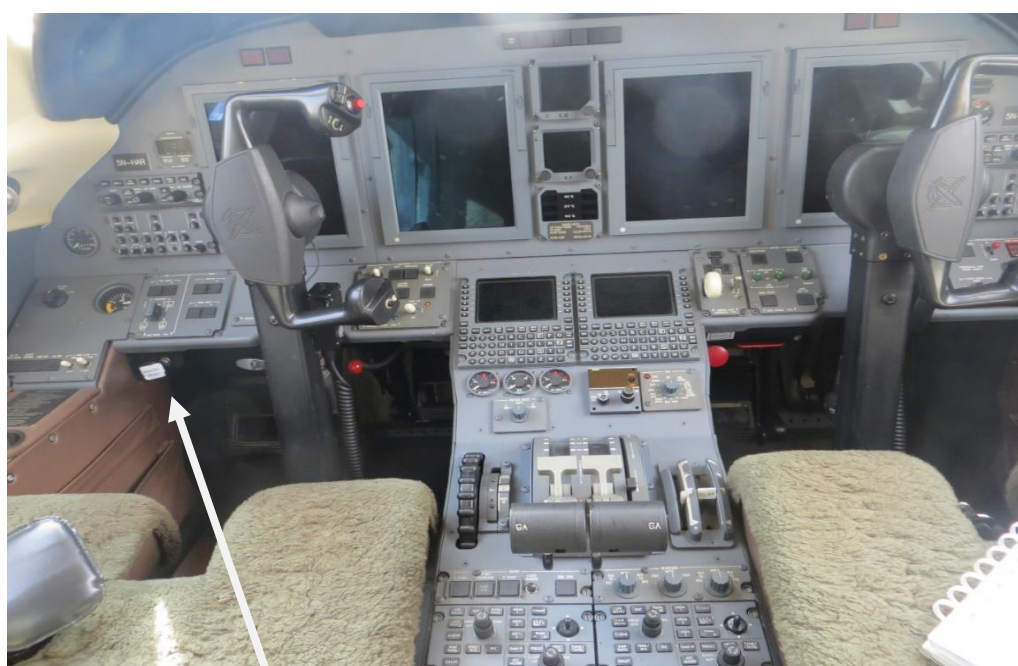
Figure 2: Parking brake position in the cockpit
