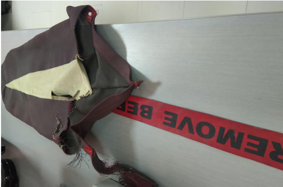
Figure 4: The severed tie-down sock from the parked Bell 412 (5N-LEH)
