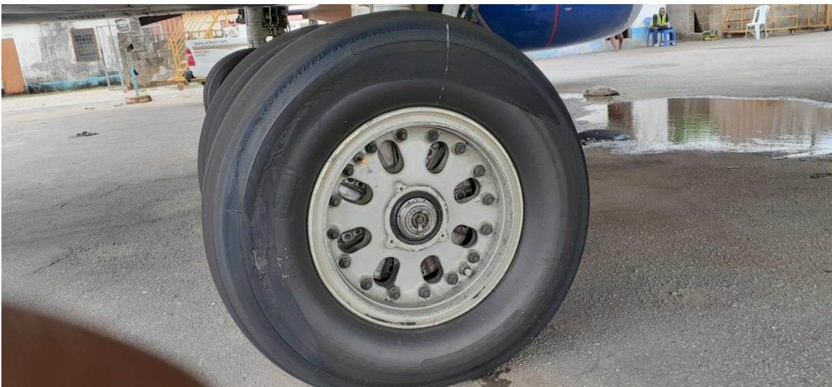
Figure 3: Photo of scuff marks on the No. 4 main wheel tyre
