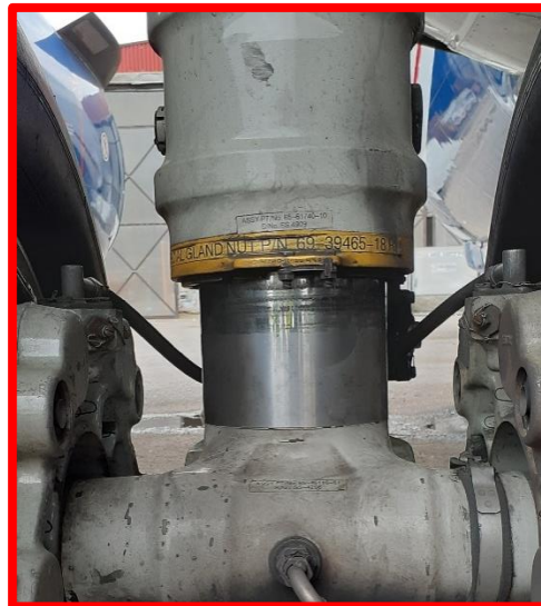
Figure 5: Photo and close up of the left main landing gear oleo strut
