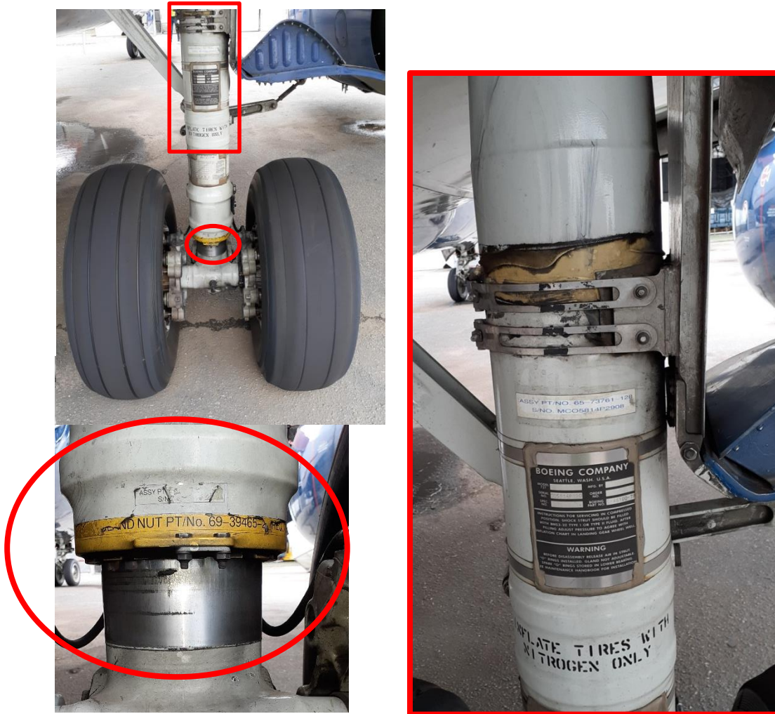
Figure 4: Photo of the displacement of the right main landing gear door clamps and oleo struts
