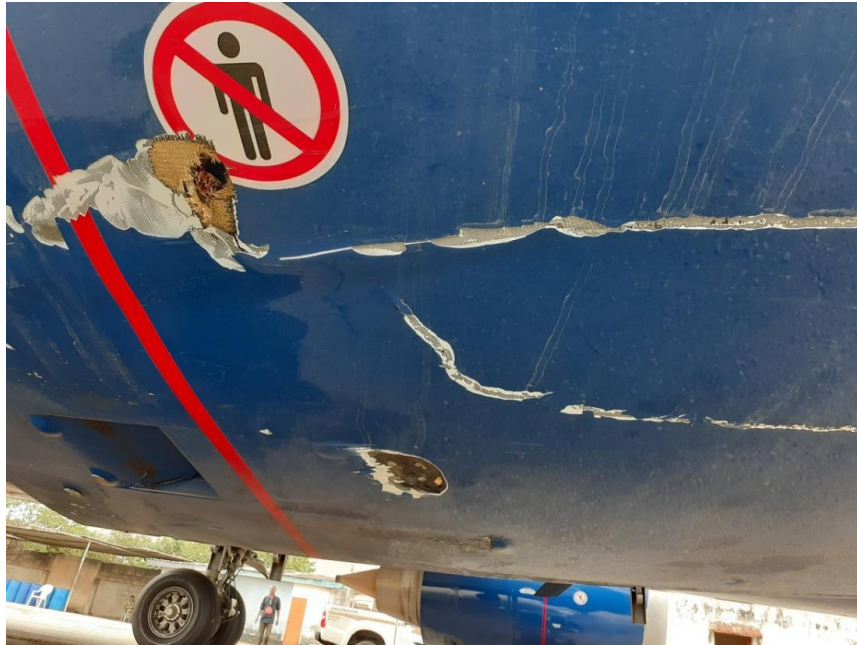
Figure 6: Photo of abrasions and dents on the No. 2 engine cowling
