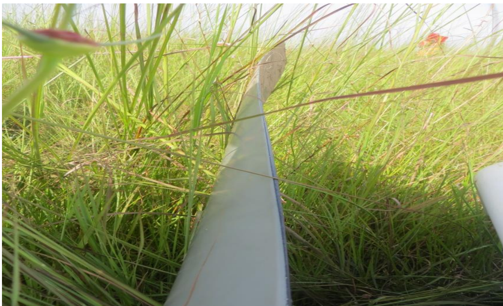
Figure 5: Damaged propeller blade.
