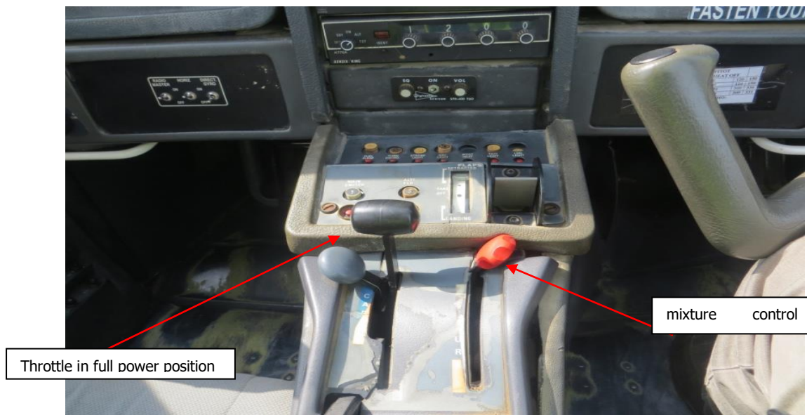
Figure 2: Engine Control Levers with throttle at FULL power position and Fuel Mix Lever at RICH position after the incident.
