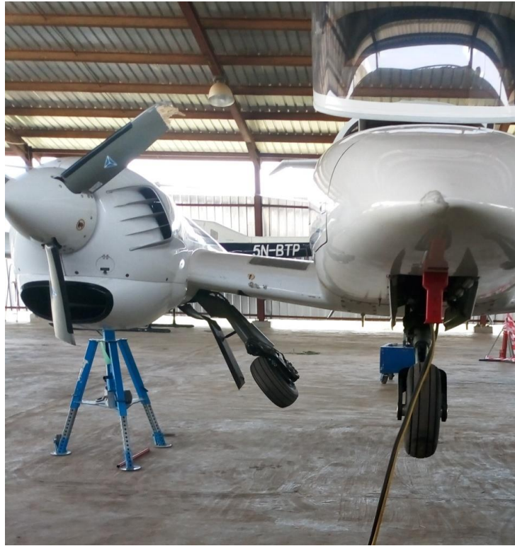
Figure 2: Photo of aircraft landing gear being retracted and extended under test
