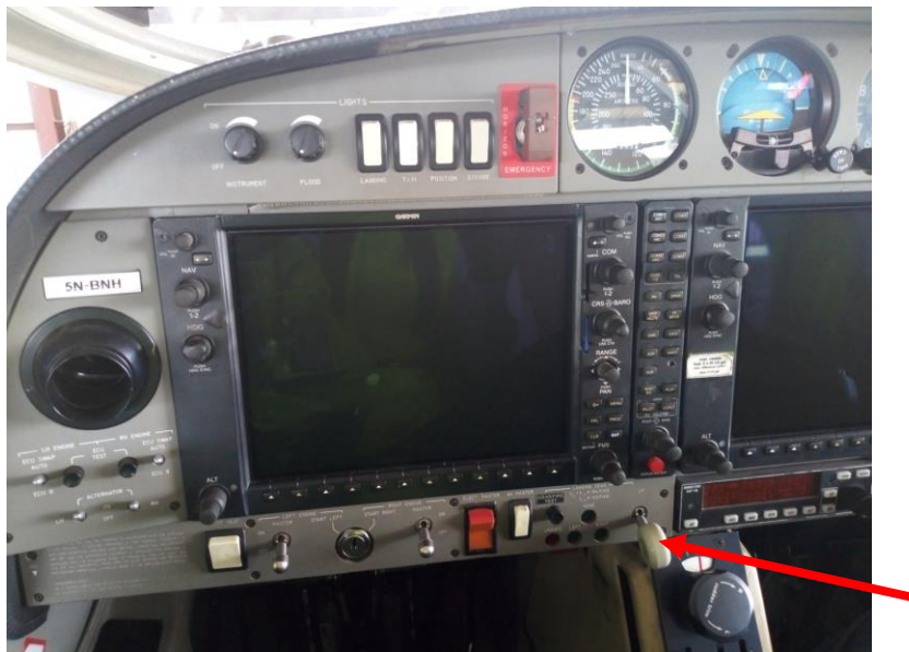
Figure 3: Photo of the knob on the landing gear switch
