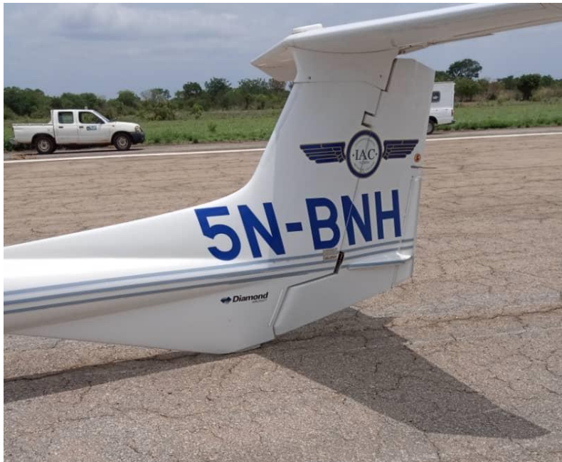
Figure 6: Photo of the tail skid of aircraft resting on the runway
