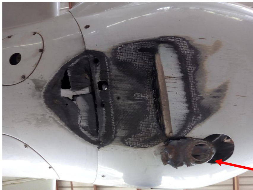
Figure 5: Photo of the base of engine cowling and exhaust abraded after the incident
