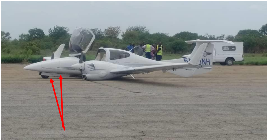
Figure 8: Photo of the nose-wheel door opened and landing gear partially extended
