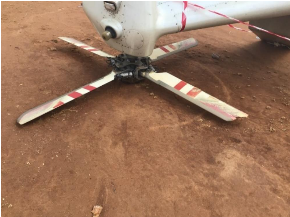
Figure 11: Damaged tail rotor blades
