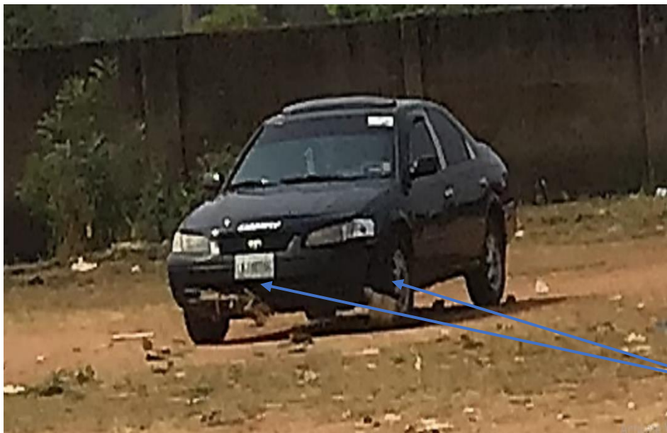
Figure 2: Damage to a parked car from flying debris
