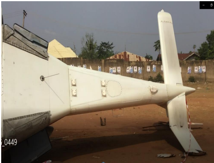
Figure 9: Damaged right horizontal stabilizer
