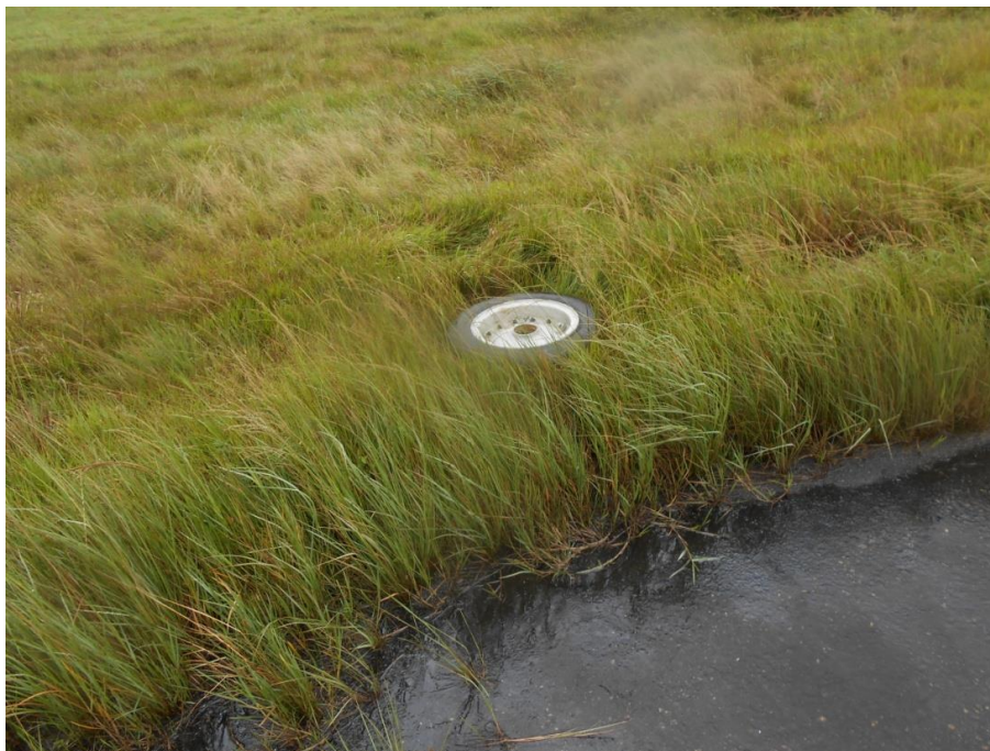
Figure 10: Photo showing LH nose wheel assembly found outside the runway on the grass verge, 1,058 m from the threshold
