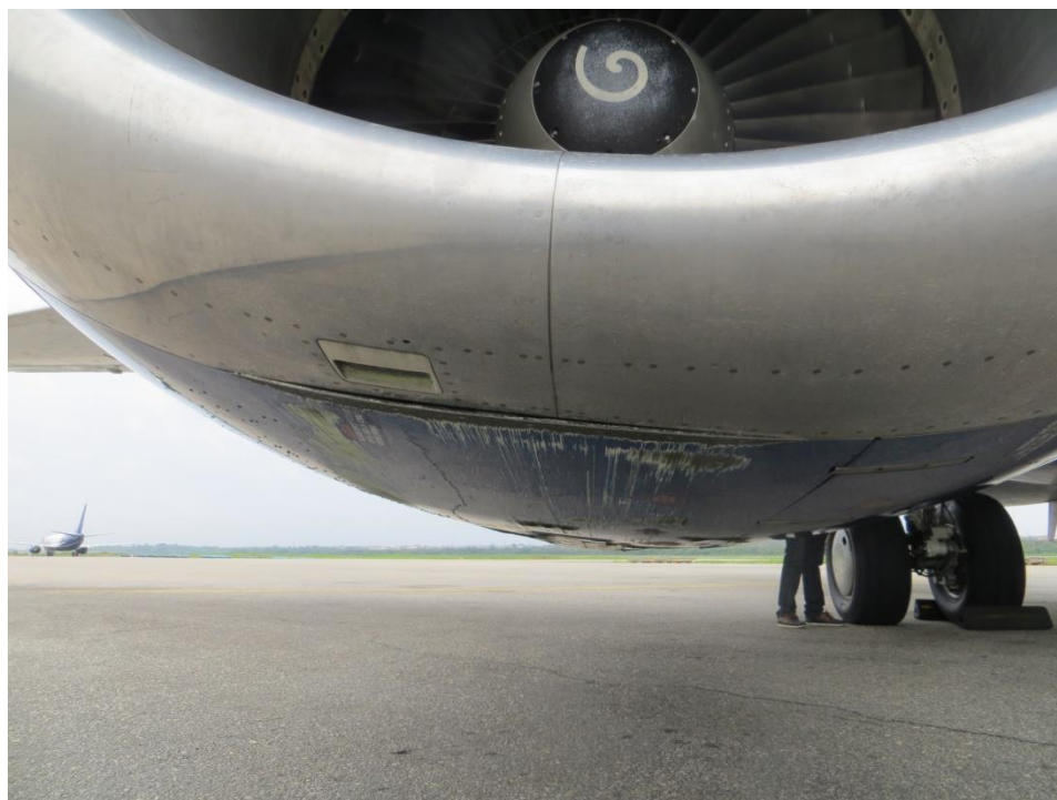
Figure 12: Photo showing the damage to lower fan cowl of RH Engine
