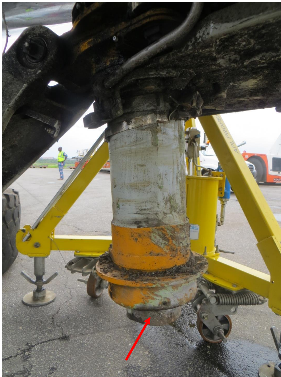
Figure 7: Photo indicating 0.984 inches of the remains of the nose landing gear shock strut
