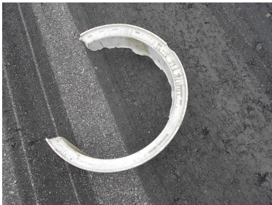
Figure 8: Photo showing flange of the RH nose wheel assembly found at 971 m from runway threshold
