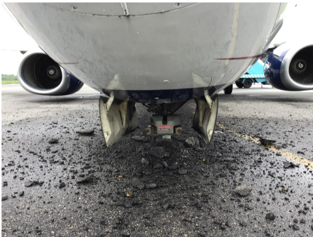
Figure 5: Photo showing nose landing gear strut stuck in the runway
