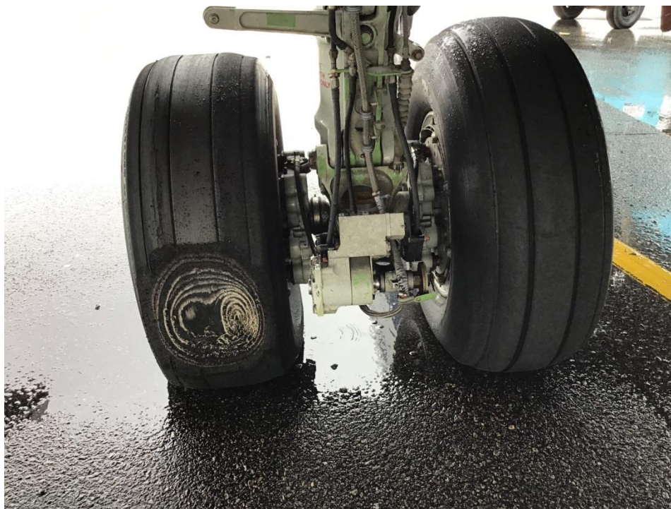
Figure 11: Photo showing severe flat spot on the deflated RH main wheel outboard tyre
