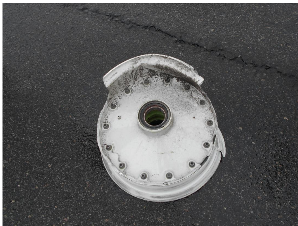
Figure 9: Photo showing the main half of the RH nose wheel assembly found 1,129 m from the threshold
