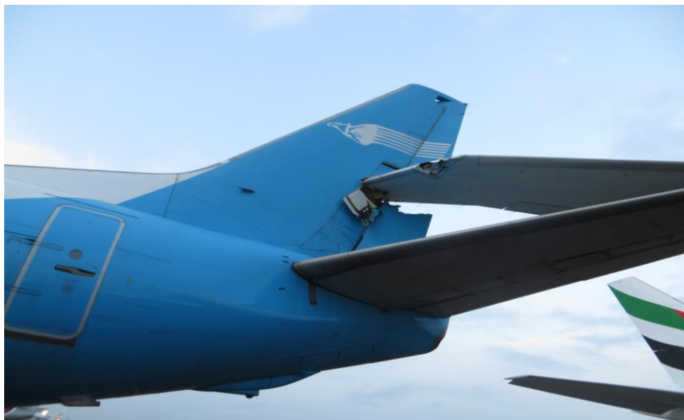
Figure 5: Another close-up view of the damage to the rudder and the tail section of 5N-BOU
