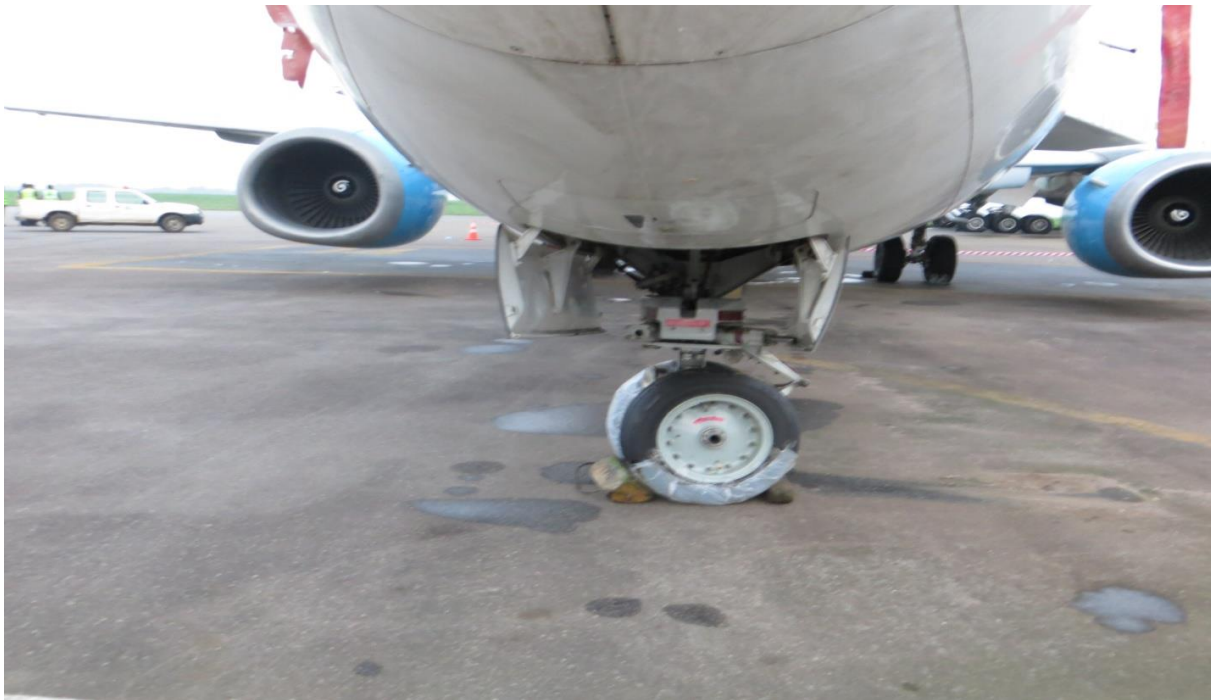
Figure 7: HAK Air Nose wheel at 90° due to the impact with Emirates aircraft
