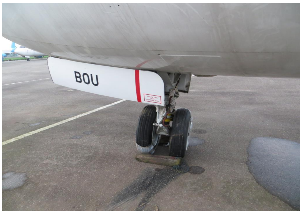
Figure 6: HAK Air Aircraft moved 5ft sideways and nose wheel turned 90°
