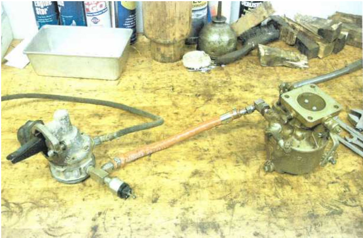
Fig. 1-13 showing hose connecting the fuel pump that supplies fuel to the Carburetor
