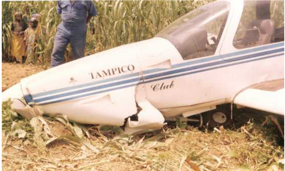
Fig. 1.12a Photograph showing nose landing gear sheared off from its attachment point
