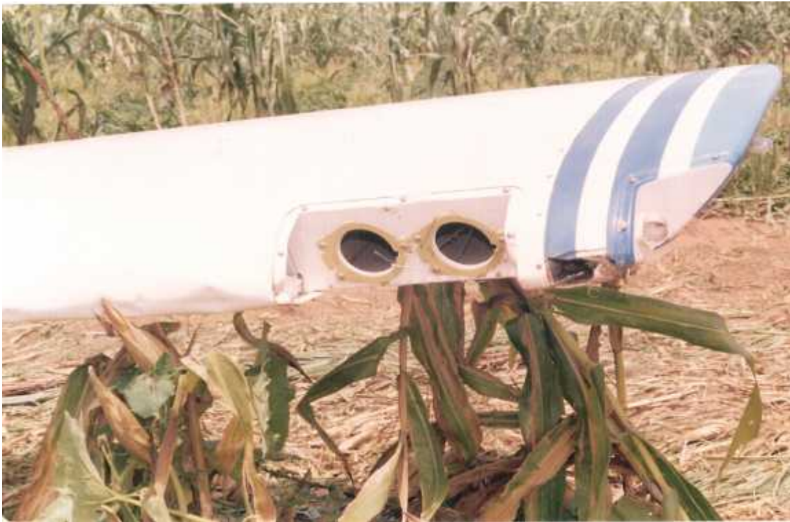
Fig. 1.12.1 Photograph showing right wing taxi and landing light destroyed
