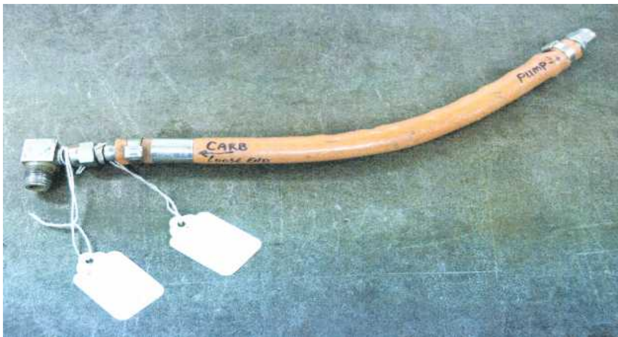
Fig. 1-12 showing loose and cross threaded 90° ends of the fuel hose.
