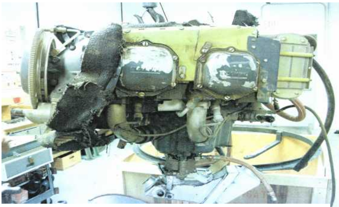
Fig.1-8 Photograph showing 5N-CBF Engine 0320-D2A in the facility of Lycoming USA for Tear Down/Stripping
