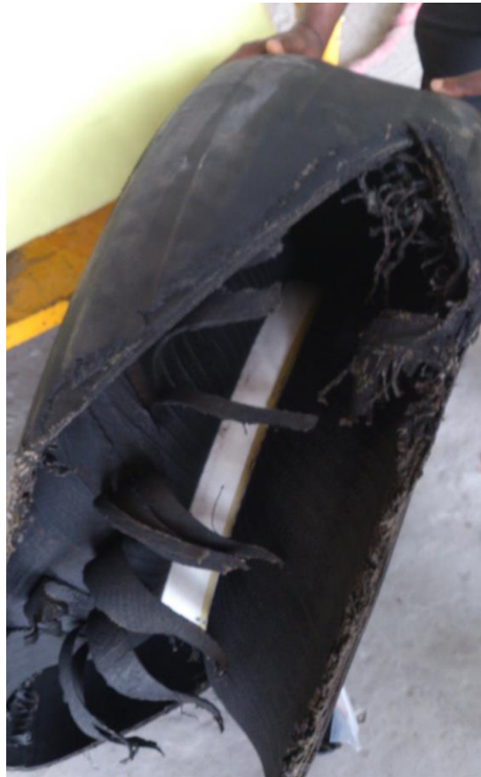
Figure 9: Damage to tyre of No. 4 Main landing Gear
