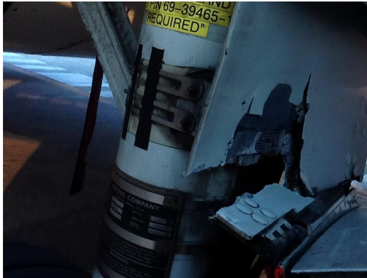
Figure 3: Damage to No. 4 Main landing gear strut and doors
