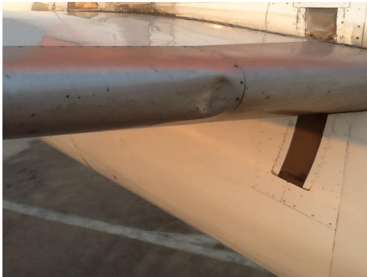
Figure 2: Damage to the leading edge of horizontal stabilizer
