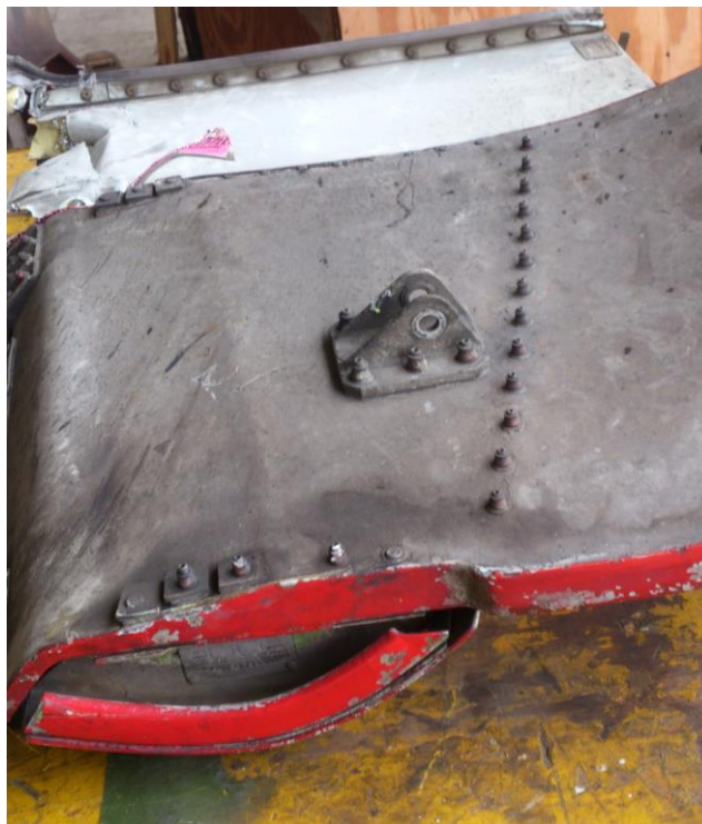
Figure 6: Damage to the wheel well doors
