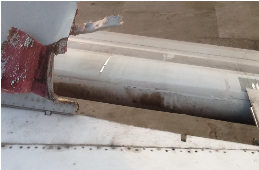
Figure 5: Damage to the edges of the Vertical/Horizontal Stabilizers
