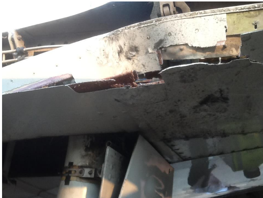
Figure 4: Damage to No. 4 Main landing gear struts and doors
