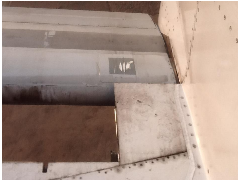
Figure 7: The missing section of the right wing
