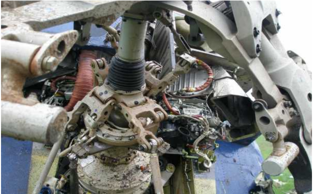
Photograph showing rotor assembly and transmission damage
