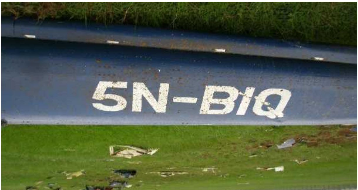
Photograph showing separation of tail boom
