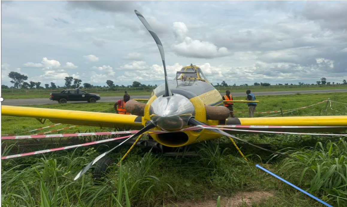
Figure 5: The bent propeller blades and the stuck left main landing gear
