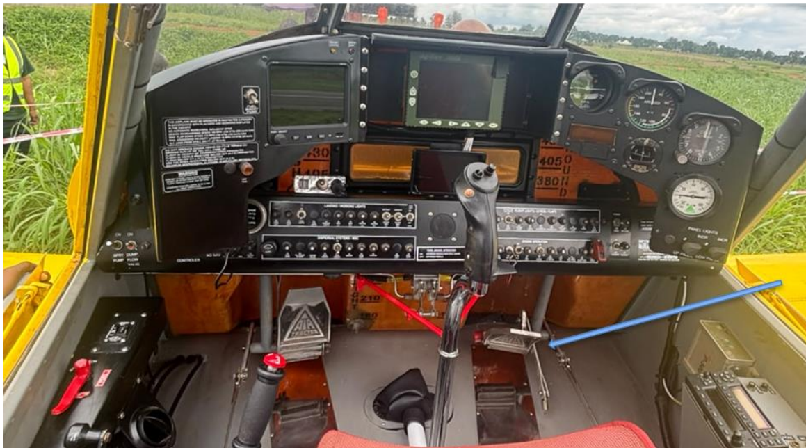
Figure 6: Right rudder-pedal linkage found work loosen at the attachment.
