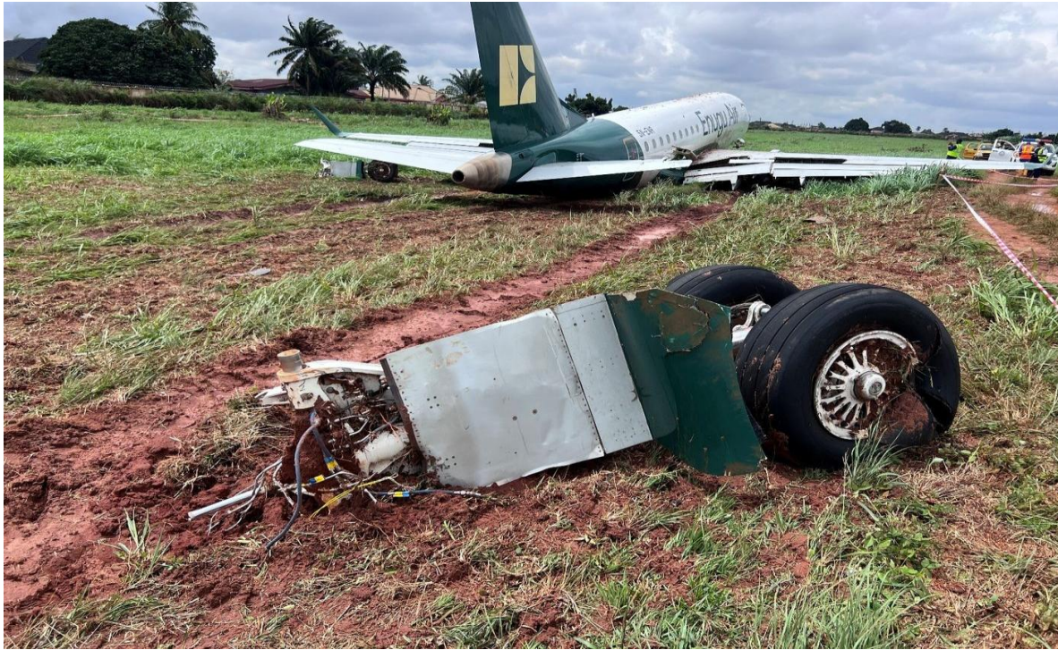
Figure 10: Separated right main landing gear assembly
