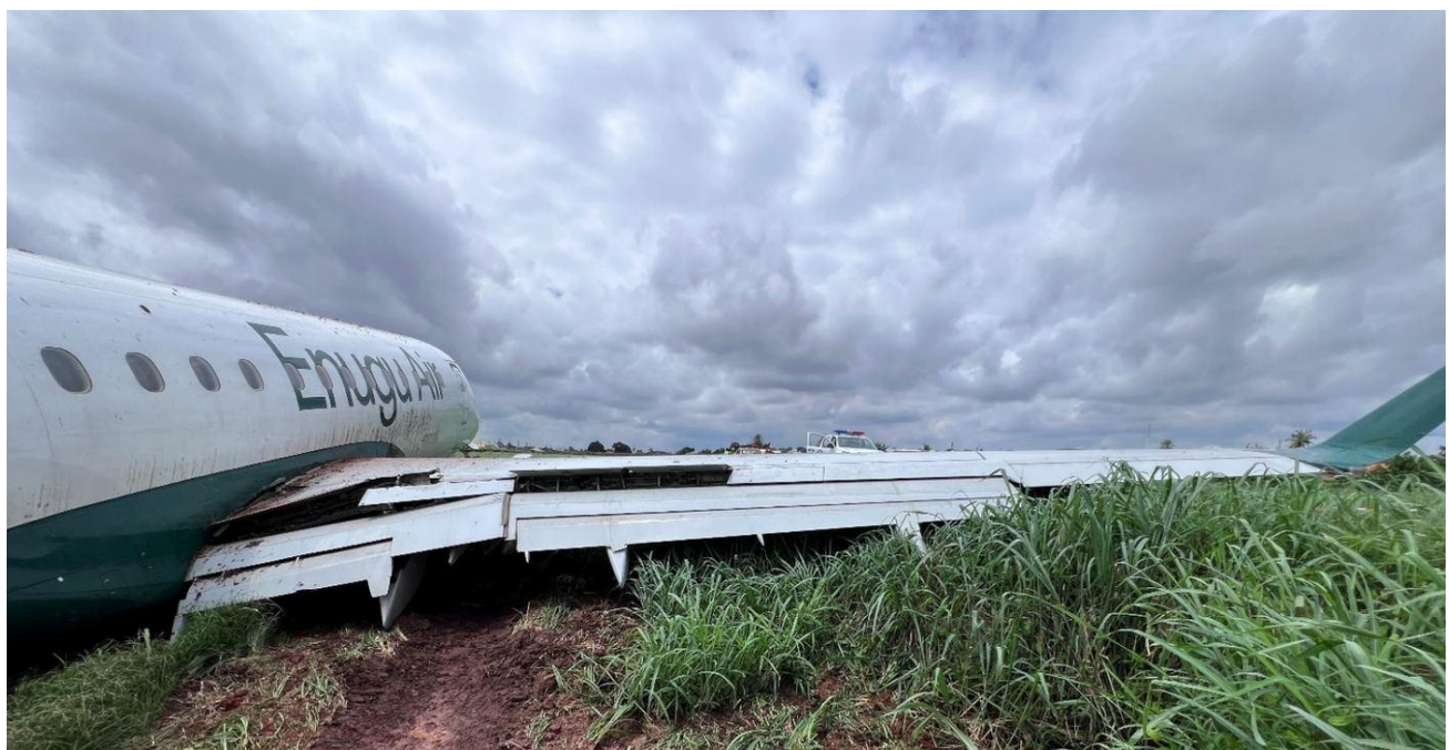
Figure 21: The ruptured right wing aileron and flaps
