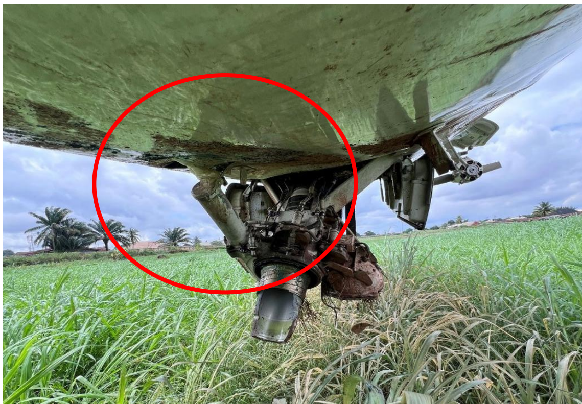
Figure 15: Ruptured forward lower fuselage skin
