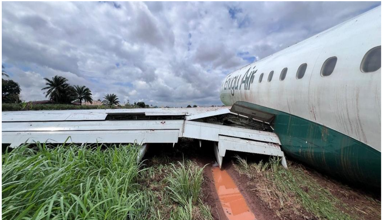
Figure 20: The ruptured left wing aileron and flaps
