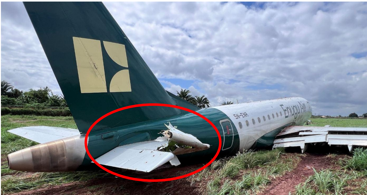
Figure 14: Ruptured horizontal stabilizer
