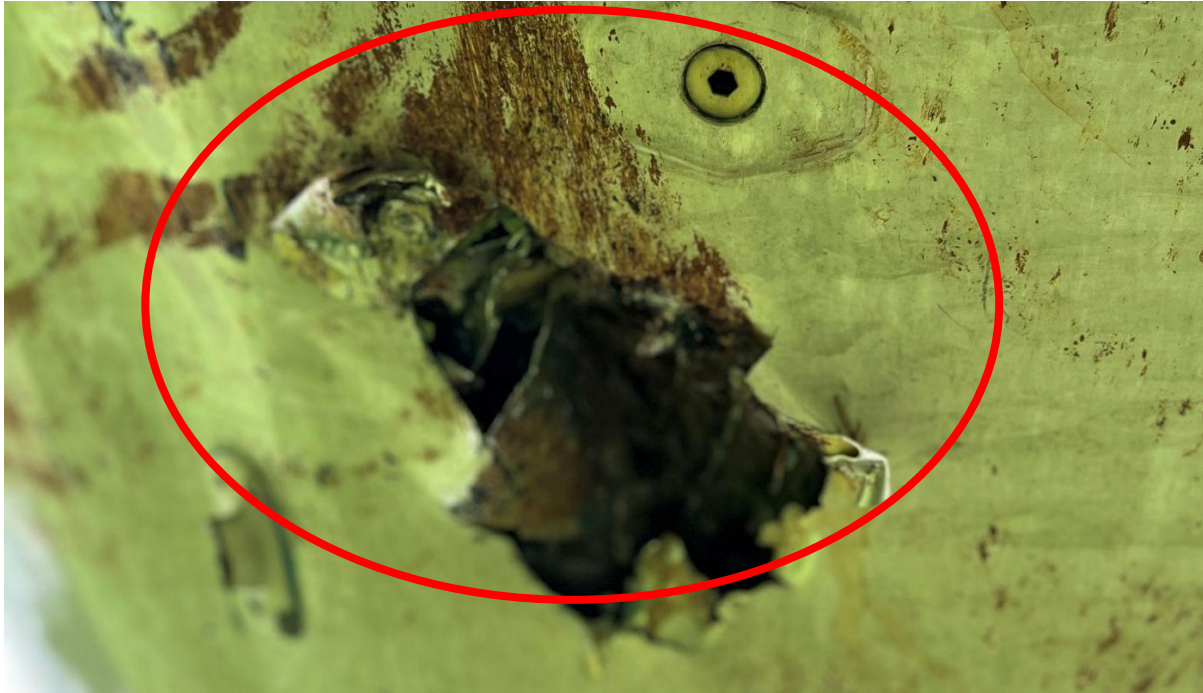
Figure 16: Close-up of the ruptured forward lower fuselage skin.
