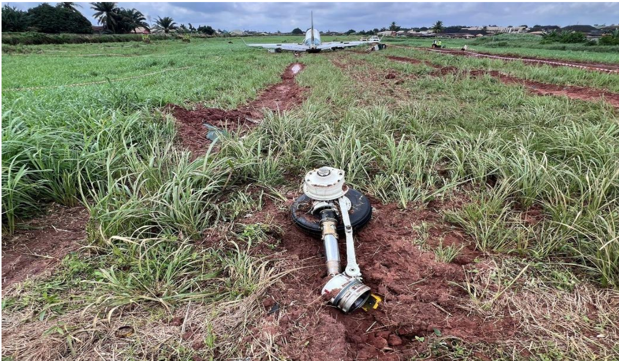
Figure 9: Separated nose landing gear assembly
