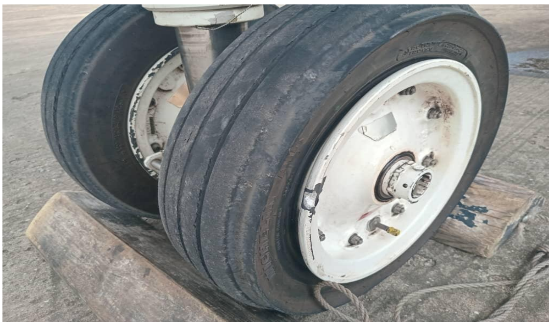
Figure 1: Damage to the left nose-wheel assembly identified during post-flight inspection.
