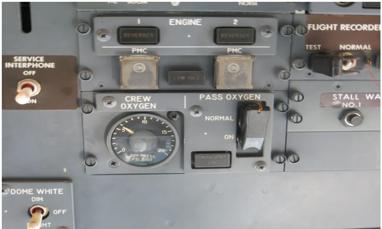
Figure 4: The passenger oxygen switch in normal position and wire-locked during post occurrence inspection
