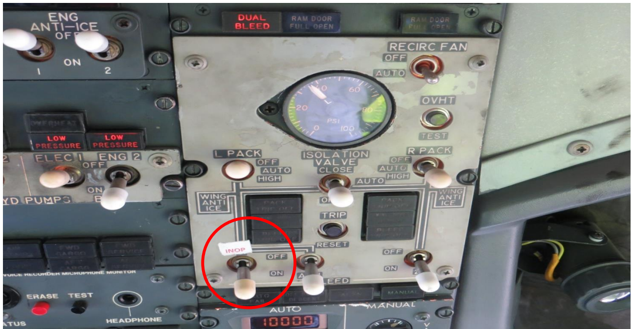
Figure 3: The left engine bleed switch on air-conditioning control panel with 'INOP' placard
