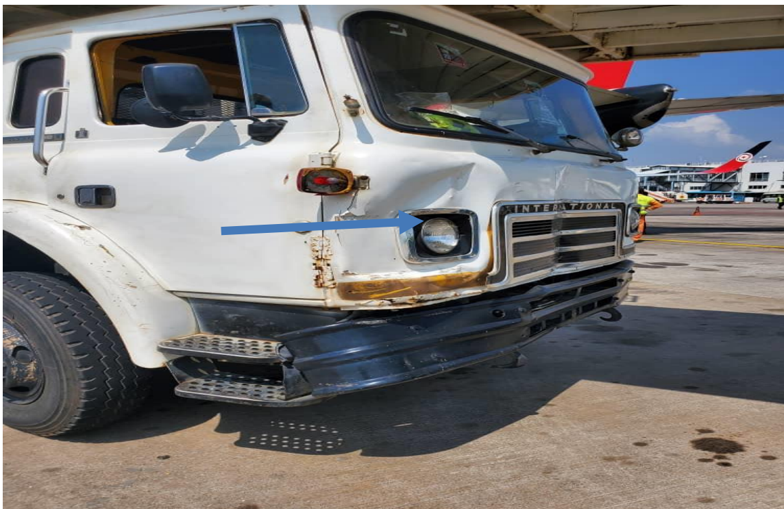
Figure 8: Dent on the catering service truck.
