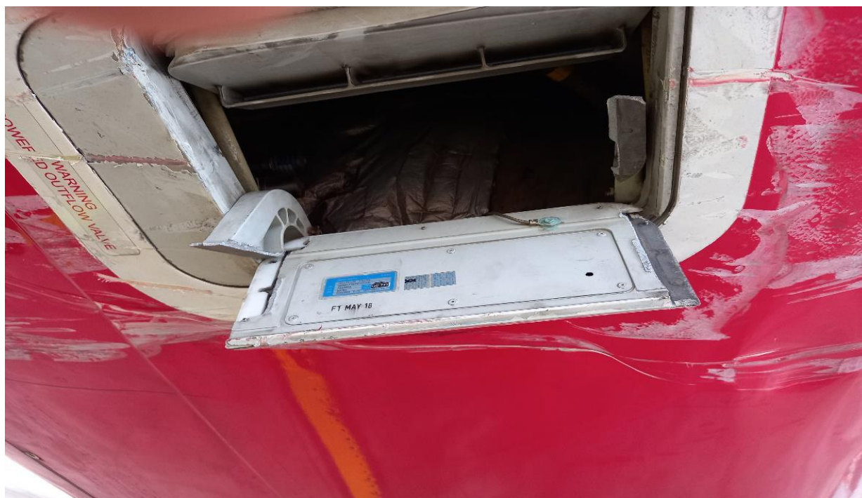
Figure 6: Broken outflow valve.
