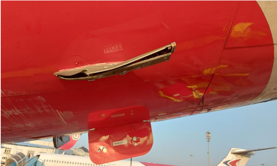
Figure 3: Dent around the rear pressure bulkhead area.
