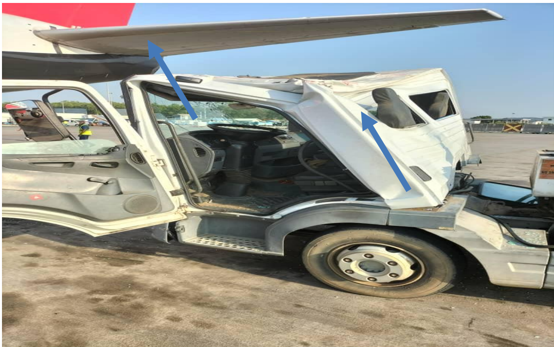
Figure 7: Damaged lavatory service truck after the incident.
