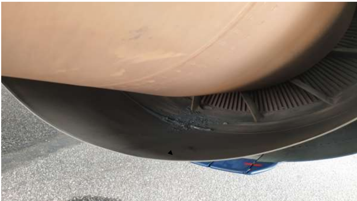
Figure 2: Metal debris in the tail cone of No. 2 engine during post occurrence inspection
